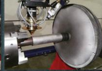
Laser cladding & hardening is a technology used to restore the service life of various critical components used in the shipping industry, the energy industry, the heavy industry, refineries etc, such as:
