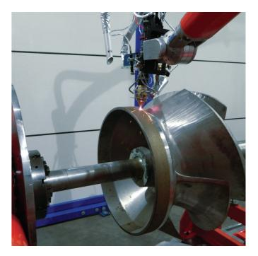
For more than twelve years, KIMI has applied advanced laser cladding technique for repair welding and hardening that recovers and prolongs the lifecycle of high value machinery components. The laser beam creates a shallow molten pool at the workpiece to which a filler material is fused. The bond created between the fused powder and the base metal is metallurgical.
